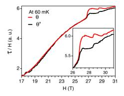
Fig. 6: (Colour on-line) Dzyaloshinski-Moriya contribution within the 1/8 plateau and its adjacent phase. Torque data have been recorded at  $\theta = +0.4^{\circ}$  and at  $-|\theta'|$ . The latter data have been rescaled to give the same signal at 17 and 26 T. Two signals strongly differ within the plateau and its adjacent phase, which is attributed to a symmetry breaking.
