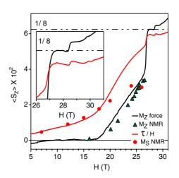
Fig. 4: (Colour on-line) Comparison of torque and magnetization. Magnetization was measured both by NMR technique, green triangles, and by torque in a field gradient, continuous black line. Those measurements are compared with torque divided by field, the continuous red line. The solid red circles correspond to the transverse staggered magnetization measured by <sup>11</sup>B NMR.
