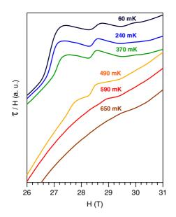
Fig. 3: (Colour on-line) Torque divided by field vs. field at different temperatures. The measurements were made for field sweep up. The curves have been arbitrary shifted for clarity.
