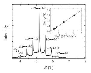
Fig. 8. Field swept NMR spectrum at the  $^{139}$ La sites at 6 K and 31 MHz in the magnetic field parallel to the c-axis. The inset shows the  $\delta \nu / \nu_0$  versus  $1/\nu_0^2$  plot at 115 K.
