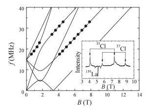
Fig. 7. Frequency-field diagram at 3 K at the <sup>35</sup>Cl sites in the applied magnetic fields *B* parallel to the *c*-axis. The solid lines show the fit obtained from the Hamiltonian (2). The inset shows the Cl-NMR spectrum at 31 MHz.
