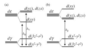
Fig. 15. Orbital energy levels for  $Cu^{2+}$  in a tetragonal crystal field. The ground state wave function is  $d(x^2 - y^2)$  in (a) or  $d(3z^2 - r^2)$  in (b).
