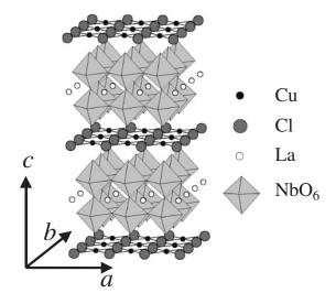
Fig. 1. Schematic drawing of the crystal structure of (CuCl)LaNb<sub>2</sub>O<sub>7</sub>.
