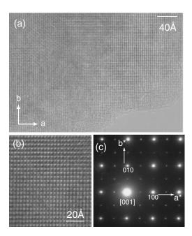
Fig. 14. (a) High-resolution TEM image of (CuCl)LaNb<sub>2</sub>O<sub>7</sub> at room temperature along the [001]-zone axis and (b) its enlarged view. (c) Corresponding electron diffraction pattern, where indices are given based on the tetragonal unit cell of the P4/mmm structure.<sup>7)</sup>
