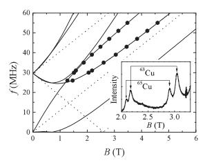
Fig. 6. Frequency–field diagram at 3 K at the  $^{63}\text{Cu}$  sites in the applied magnetic fields B parallel to the c-axis. The dotted lines represent the resonance modes for the case of axially symmetric EFG around the c-axis. The solid lines are the fit to the results obtained from the Hamiltonian (2). The inset shows the Cu-NMR spectrum at 43 MHz.
