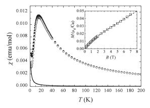
Fig. 3. Temperature dependence of  $\chi$  measured for the unaligned powder sample at 1 T. The solid circles represent the raw data. The open circles represent  $\chi$  after subtracting the impurity contribution shown by the solid line. The inset shows the magnetic field (*B*) dependence of the magnetization at 2 K. The dashed line is the fit to the form  $M = NgS\mu_B B_S(x) + AB$ .
