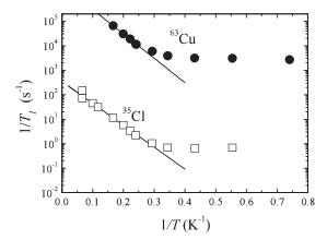
Fig. 5. Inverse temperature dependence of  $1/T_1$  at the <sup>63</sup>Cu and <sup>35</sup>Cl sites. The solid lines show the fit to an activation law  $1/T_1 \propto \exp(-E/k_BT)$ .
