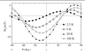
**Figure 2.** Angular variation of  $H_1$  at different temperatures in the external field of 6.948 T.
