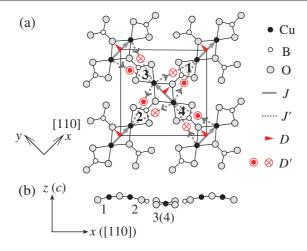
**Figure 1.** The magnetic layer of  $SrCu_2(BO_3)_2$  viewed along (a) the c-(z-) and (b) the  $[1\overline{1}0]$ -(y-) directions. Numbers are the site indices for both Cu and B. Symbols for D and D' indicate the direction of d in the Dzyaloshinsky–Moriya interaction  $d \cdot (s_i \times s_j)$  with the bond direction  $i \to j$  shown by arrows.
