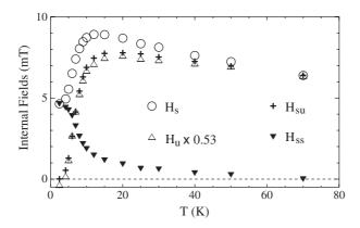
**Figure 3.** Temperature dependences of  $H_u$ ,  $H_s$ , (4)  $H_{su}$ , and  $H_{ss}$  (6) at  $H_{ext} = 6.948$  T.
