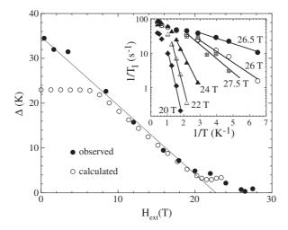
**Figure 5.** Field dependence of the excitation gap (solid circles in the main panel) determined from the activated behaviour of  $1/T_1$  (inset) compared with the results of ED calculation (open circles). The data at 27.5 T, where the NMR spectrum shows many lines in the 1/8-plateau phase, were obtained for the line with the largest (negative) hyperfine field.
