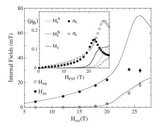
**Figure 4.** Field dependences of  $H_{\rm Su}$  and  $H_{\rm SS}$  measured at low temperatures, 2.5 K (for  $H_{\rm ext}=7$  and 12 T), 1.5 K (15 and 17.9 T), 0.64 K (20 T), 0.46 K (24 T), and 0.21 K (26 T). The curves are obtained from the ED results of  $\sigma_x$ ,  $\sigma_z$ ,  $M_z$ , and  $M_x^{\rm A,B}$  shown in the inset by using (7) and (8).
