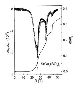
Fig. 1. Relative change of the elastic constant  $c_{11}$  in SrCu (BO<sub>3</sub>)<sub>2</sub> for the magnetic field sweep up (solid circles) and sweep down (open circle) measured at T = 1.5 K. Field dependence of relative magnetization  $m/m_0$  at the same temperature is also shown (solid line). Here  $m_0$  is a saturation value of the magnetization. The magnetic field applied along the a - axis. The elastic constant minima occur between the magnetization plateaus.
