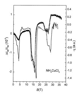
Fig. 2. Magnetic field dependence of the transversal mode  $c_{66}$  together with the magnetic susceptibility form Ref. [9]. (solid line) for NH<sub>4</sub>CuCl<sub>3</sub>. Both measured at T = 1.5 K. For the elastic constant only the magnetic field sweep down (open circles) is shown. The external magnetic field is applied parallel to the a - axis.
