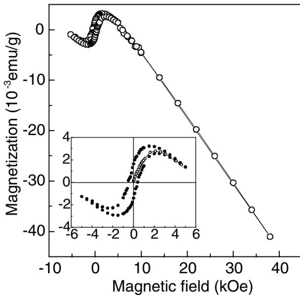
Fig. 4. Field dependence of PbTe:0.3 at.%Ga magnetization at  $T = 5$  K. The inset shows the hysteresis in a low magnetic field.
