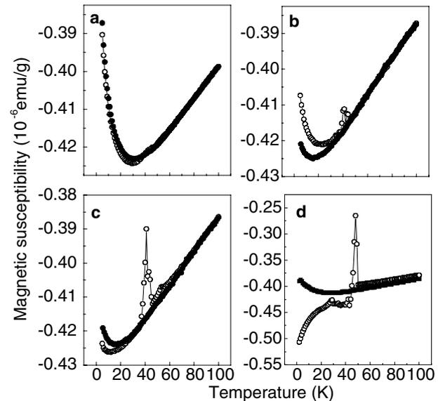
Fig. 3. Temperature dependencies of magnetic susceptibility of  $\text{PbTe}:0.3$  at.%Ga both upon heating (open circles ○) and cooling (solid circles ●) measured in the dark chamber of SQUID magnetometer after different exposures to white-light illumination ( $t_{\text{exp}}$ ) at room temperature. (a)  $t_{\text{exp}} = 5 \times 10^2$  sec; (b)  $t_{\text{exp}} = 5 \times 10^3$  sec; (c)  $t_{\text{exp}} = 1.5 \times 10^4$  sec; (d)  $t_{\text{exp}} \geq 10^5$  sec.
