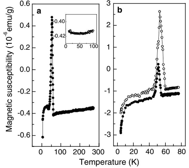
Fig. 2. Temperature dependencies of magnetic susceptibility upon heating after brief illumination at low temperature. (a)  $\text{PbTe}:1$  at.%In; (b)  $\text{Pb}_{0.75}\text{Sn}_{0.25}\text{Te}:0.5$  at.%In (solid circles ●) and  $\text{Pb}_{0.75}\text{Sn}_{0.25}\text{Te}:2$  at.%In (open circles ○). The inset in panel (a) shows the temperature dependence of the magnetic susceptibility of the undoped sample of PbTe.
