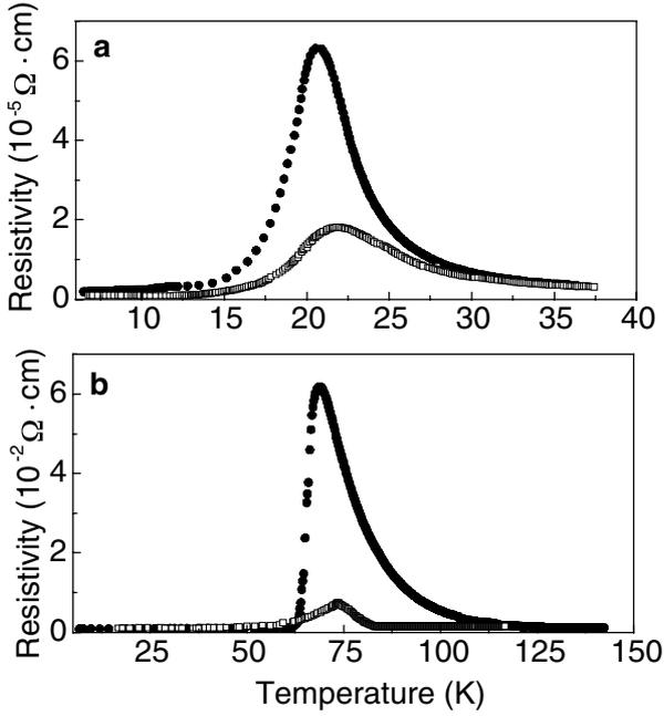
Fig. 1. Temperature dependencies of resistivity upon heating after brief illumination at low temperature (solid circles ●) and under permanent illumination (open squares □). (a)  $\text{Pb}_{0.75}\text{Sn}_{0.25}\text{Te}:0.5$  at.%In; (b)  $\text{PbTe}:0.3$  at.%Ga.
