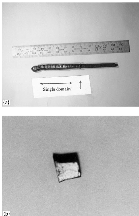
Fig. 1. The representative photos of a crystal rod (a) and a single domain (b) of  $\text{SrCu}_2(\text{BO}_3)_2$ . The upward arrow in (a) indicates the starting point of the crystal growth.
