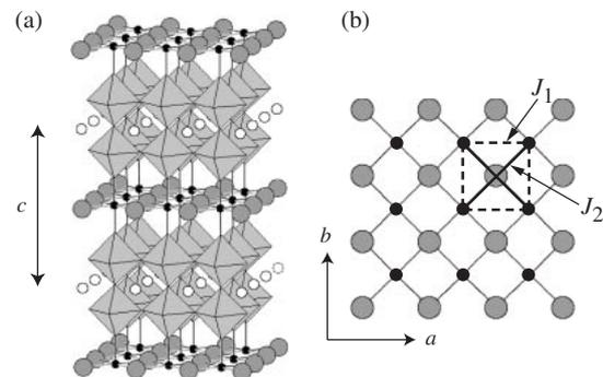
Fig. 1. (a) Schematic representation of structure of (CuCl)LaNb<sub>2</sub>O<sub>7</sub>. The closed spheres are coppers, the gray spheres are chlorines, the open spheres are lanthanums, and the octahedra are NbO<sub>6</sub> octahedra.<sup>7)</sup> (b) Copper-chlorine layer viewed along  $c$ -axis. The bold broken and solid lines represent, respectively, the  $J_1$  and  $J_2$  bonds.
