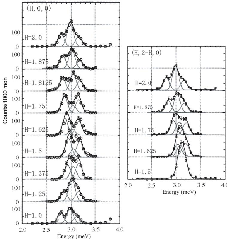
Fig. 4. Series of high-resolution energy scan at  $T = 1.5$  K for different  $Q$ . Note, that the spectrum at  $Q = (1,0,0)$  shows a three peak, at  $Q = (1.5,0,0)$  a two peak and at  $Q = (1.5,0.5,0)$  a single peak structure.
