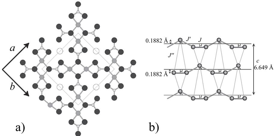
Fig. 1. (a) The structure of  $\text{SrCu}_2(\text{BO}_3)_2$  projected on  $ab$ -plane. The open circles denote  $\text{Sr}^{2+}$ , black circles  $\text{O}^{2-}$ , large grey circles  $\text{Cu}^{2+}$  and small grey circles  $\text{B}^{3+}$  ions. (b) The buckling of the dimer plane.
