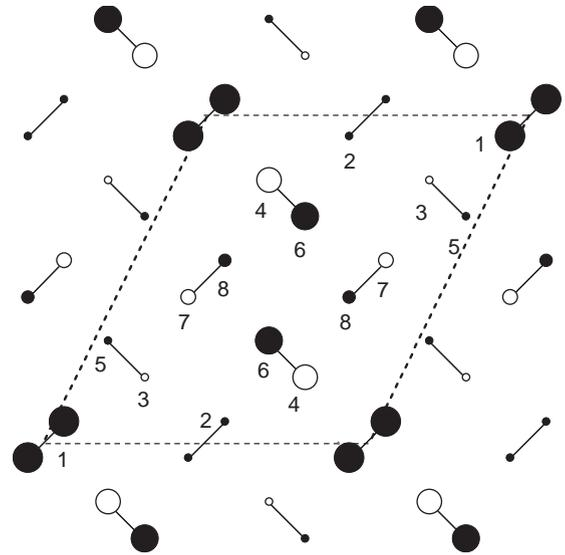
Fig. 2. Magnetization profile in the  $\frac{1}{8}$  plateau state. Closed (open) circle shows the positive (negative)  $\langle S_z \rangle$ . The circle size represents the magnitude of  $\langle S_z \rangle$ .
