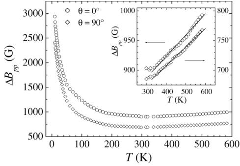
FIG. 2. Temperature dependence of the linewidth of the X-band ESR spectra of  $\text{SrCu}_2(\text{BO}_3)_2$  single crystal for  $\mathbf{B}_0 \parallel \mathbf{c}$  (circles) and  $\mathbf{B}_0 \perp \mathbf{c}$  (diamonds). Inset shows the high- $T$  linearly increasing behavior.
