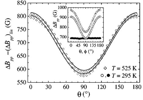
FIG. 3. X-band ESR anisotropy of  $\text{SrCu}_2(\text{BO}_3)_2$  single crystal at 525 K (diamonds) and 295 K (circles) with the high- $T$  linear part subtracted. The solid lines correspond to angular dependence predicted by Eq. (4) with  $D'_\parallel = 2.4$  K and  $D'_\perp = 4.0$  K. The inset shows "raw" linewidth anisotropy in the crystal  $ac$ -plane (open symbols) at 525 K (diamonds) and in the  $ab$ -plane at 295 K (full circles).
