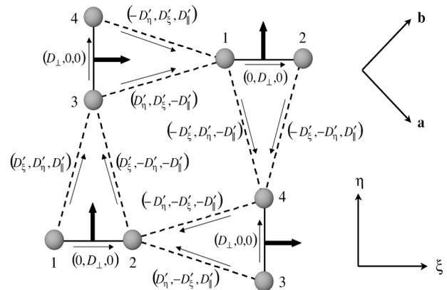
FIG. 1. The 2D network of  $\text{Cu}^{2+}$  ions with full lines representing the  $nn$  ( $J$ ) and dashed lines the  $nnn$  ( $J'$ ) exchange coupling. The interdimer  $\mathbf{D}$  and intradimer  $\mathbf{D}'$  DM interactions are also presented with the thin arrows representing the orientation of corresponding bonds for DM interaction. Thick arrows are the  $nn$  DM vectors.
