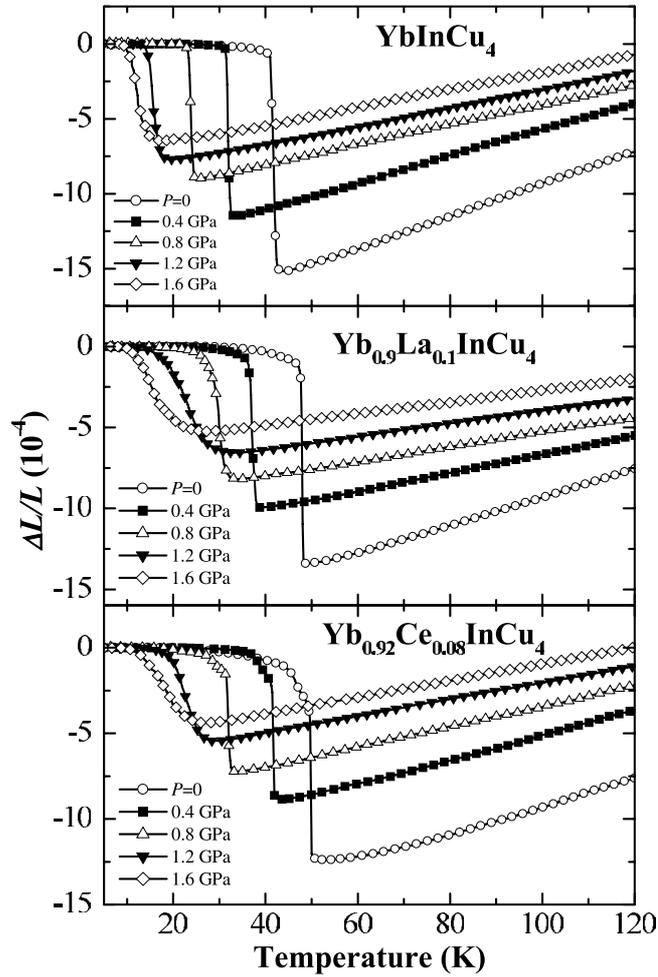
**Figure 5.** Linear thermal expansion curves of YbInCu<sub>4</sub>, Yb<sub>0.9</sub>La<sub>0.1</sub>InCu<sub>4</sub> and Yb<sub>0.92</sub>Ce<sub>0.08</sub>InCu<sub>4</sub> for different pressures.
