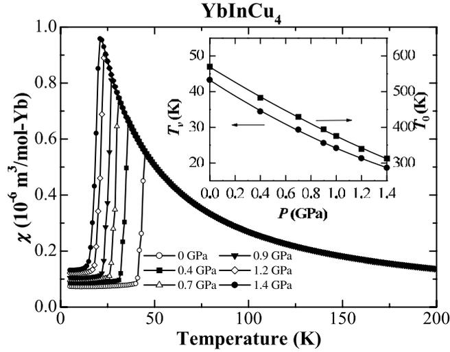
**Figure 3.** Temperature dependence of the molar susceptibility of single-crystal YbInCu<sub>4</sub> for different pressures. Inset: pressure dependence of the valence transition temperature  $T_v$  (circles) and the low-temperature Kondo scale  $T_0$  (squares) for YbInCu<sub>4</sub>.
