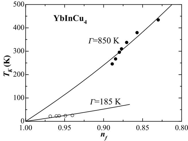
**Figure 7.** Kondo temperature  $T_K$  as a function of the 4f hole occupation  $n_f$  for YbInCu<sub>4</sub>. Closed and open circles show the data for the low- and high-temperature states, respectively. The lines represent the fits to equation (3).
