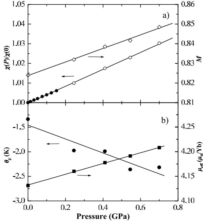
**Figure 4.** Pressure dependence of the reduced magnetic susceptibility  $\chi(P)/\chi(0)$  and the reduced effective magnetic moment  $M = \chi T/C$  at 150 K (a) and the parameters  $\theta_p$  and  $\mu_{\text{eff}}$  obtained from the Curie–Weiss fit (b) for single-crystal YbInCu<sub>4</sub>. The lines represent the linear fits to the experimental data.
