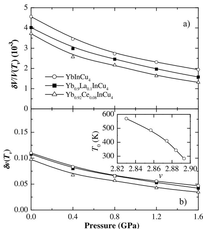
**Figure 6.** Pressure dependence of the volume (a) and valence (b) change at the valence phase transition in  $\text{YbInCu}_4$ ,  $\text{Yb}_{0.9}\text{La}_{0.1}\text{InCu}_4$  and  $\text{Yb}_{0.92}\text{Ce}_{0.08}\text{InCu}_4$ . Inset:  $T_0$  as a function of Yb valence  $v$  for  $\text{YbInCu}_4$ .
