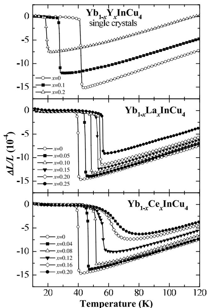
**Figure 1.** Linear thermal expansion curves of  $\text{Yb}_{1-x}\text{Y}_x\text{InCu}_4$ ,  $\text{Yb}_{1-x}\text{La}_x\text{InCu}_4$  and  $\text{Yb}_{1-x}\text{Ce}_x\text{InCu}_4$ , for different  $x$  at ambient pressure.
