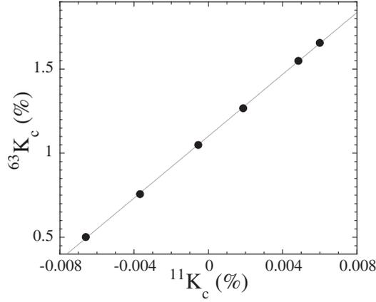
**Figure 5.** The magnetic hyperfine shift at Cu sites ( $^{63}K_c$ ) is plotted against the shift at B sites ( $^{11}K_c$ ). Both were taken at the same field,  $H = 8$  T, along the  $c$ -axis in the temperature range below 4.2 K.
