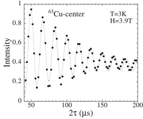
**Figure 6.** The spin-echo intensity of peak B in figure 4 for the centre line of the  $^{63}\text{Cu}$  NMR spectrum is plotted as a function of  $2\tau$ , where  $\tau$  is the separation time between  $\pi/2$  and  $\pi$  pulses. The data are taken at  $H = 3.9$  T along the  $c$ -axis and  $T = 3$  K.
