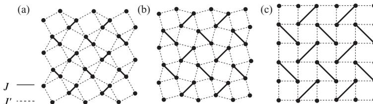
Fig. 1. Topologically identical structures realized by (a)  $\text{SrCu}_2(\text{BO}_3)_2$ , (b)  $\text{Nd}_2\text{BaZnO}_5$  and (c) Shastry-Sutherland.
