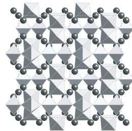
Fig. 6. Crystal structure of  $\text{KIrO}_3$ , where the  $\text{IrO}_6$  octahedra and the K ions are represented.
