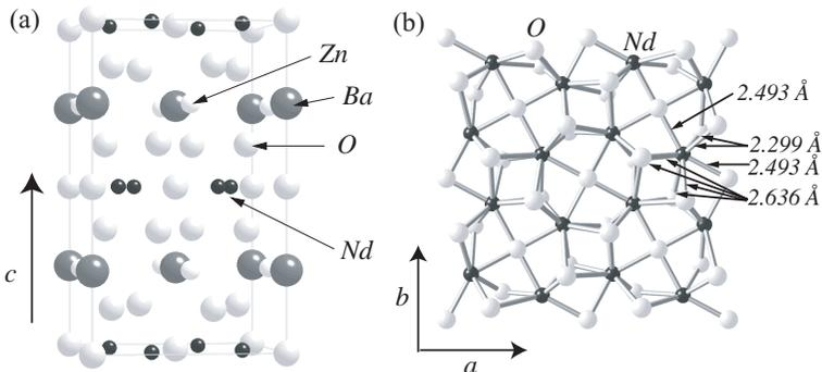
Fig. 3. Crystal structure of  $\text{Nd}_2\text{BaZnO}_5$ .
