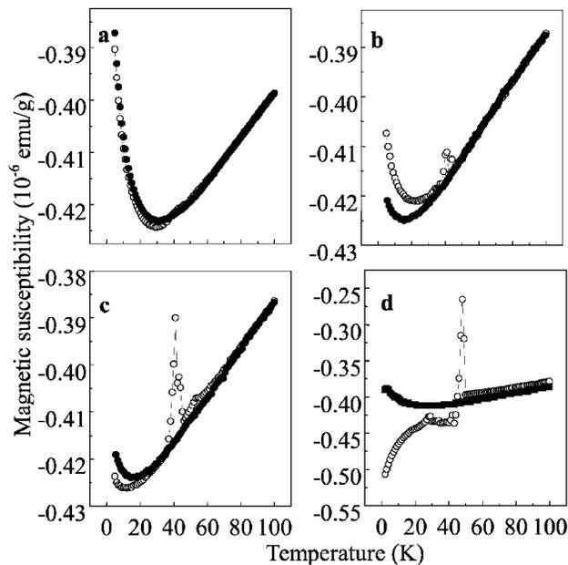
**FIGURE 3.** Temperature dependencies of magnetic susceptibility of PbTe:0.3at.%Ga both at heating (open circles) and cooling (solid circles) measured in the dark chamber of SQUID magnetometer after different exposures to white-light illumination ( $t_{exp}$ ) at room temperature. **a**,  $t_{exp} = 5 \times 10^2$  sec; **b**,  $t_{exp} = 5 \times 10^3$  sec; **c**,  $t_{exp} = 1.5 \times 10^4$  sec; **d**,  $t_{exp} = 10^5$  sec.
