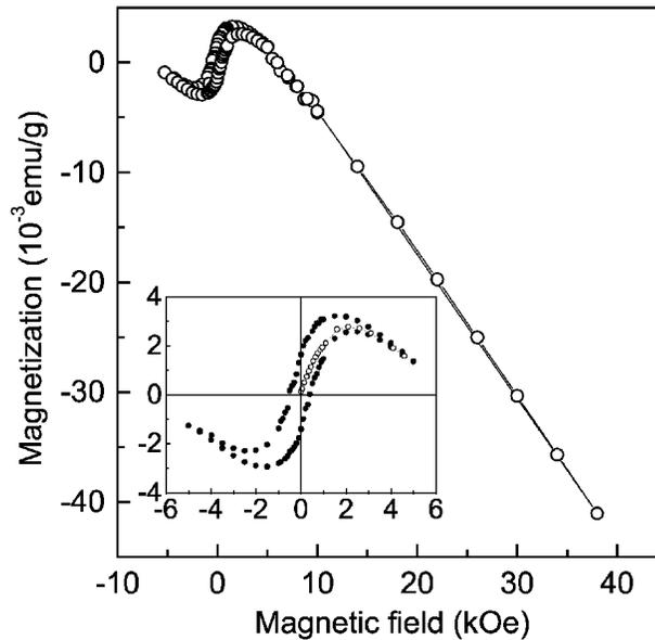
**FIGURE 4.** Field dependence of PbTe:0.3at.%Ga magnetization at  $T = 5K$ . The inset shows the hysteresis in low magnetic field.
