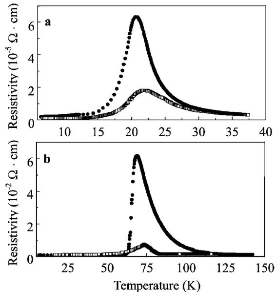
**FIGURE 1.** Temperature dependencies of resistivity at heating after brief illumination at low temperature (solid circles) and under permanent illumination (open circles). **a**,  $Pb_{0.75}Sn_{0.25}Te$ :0.5at.%In; **b**, PbTe:0.3at.%Ga.
