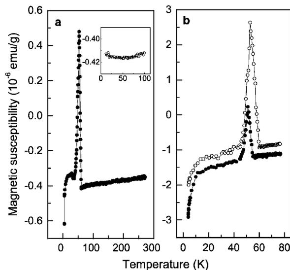
**FIGURE 2.** Temperature dependencies of magnetic susceptibility at heating after brief illumination at low temperature. **a**,  $\text{PbTe:1at.\%In}$ ; **b**,  $\text{Pb}_{0.75}\text{Sn}_{0.25}\text{Te:0.5at.\%In}$  (solid circles) and  $\text{Pb}_{0.75}\text{Sn}_{0.25}\text{Te:2at.\%In}$  (open circles). The inset to panel **a** shows the temperature dependence of the magnetic susceptibility of the undoped sample of PbTe.
